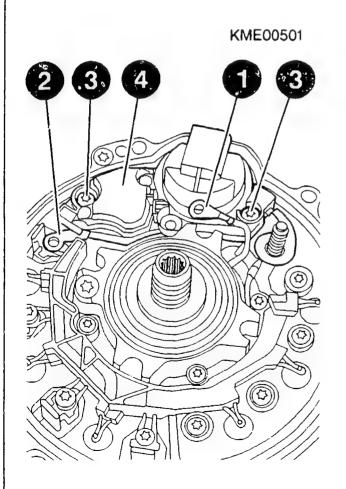
DISMANTLING AND CHECKING ALTERNATOR Dismantling regulator Detach regulator (1). NOTE: Pay attention to DF connection (2) and connection of terminal B+ (3).
